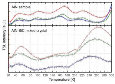
Fig. 1: TSL spectra measured at heating rates of 20 K/min (upper curve), 15 K/min (middle curve) and 10 K/min (lower curve) of a) an AlN sample with silicon and oxygen around  $1*10^{18}$  cm<sup>-3</sup> and b) and AlN-SiC mixed crystal.
